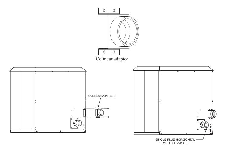
1. Attach colinear adaptor to back of heater with two (2) screws.
